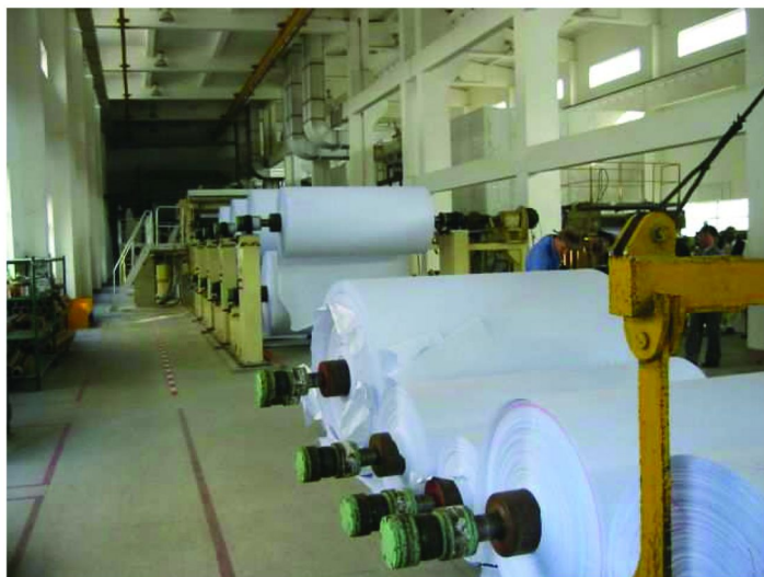
Figure 1. Bagasse paper production in a sugarcane mill in China
