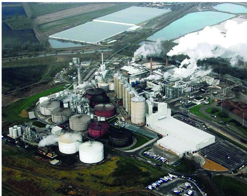
Figure 9. Wissington Sugar Factory and ethanol complex in Norfolk, UK. This is currently the largest beet biorefinery in Europe and is owned and operated by British Sugar, plc. The storage tanks allow the site to produce sugar for longer periods of time in comparison to other beet sugar factories. Additionally there is the CHP plant, the glasshouse, chromatographic separation, and ethanol production. (see color insert)
