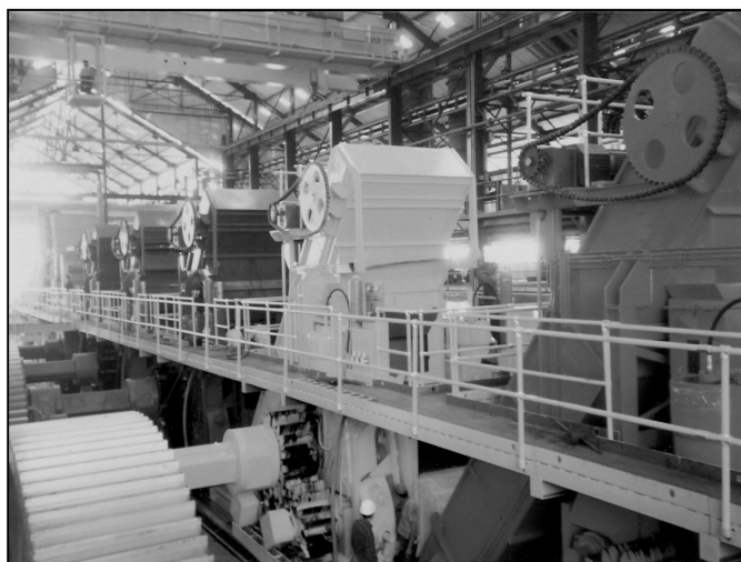
Figure 4. Tandem roller mills. Photo courtesy of Fulton Iron Works. Used with permission.
